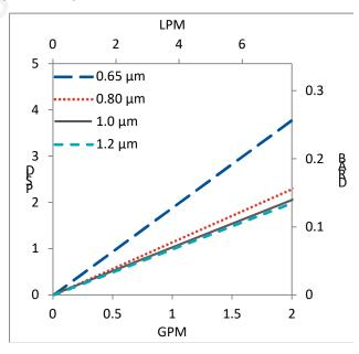
Flow rates for Capsule filters are tested using a 2" capsule filter with 1" sanitary inlet and outlet ports. The test fluid is water at ambient temperature. Flow rates for larger capsules will scale with filtration area. Rates will vary based on end configuration of the capsule.
