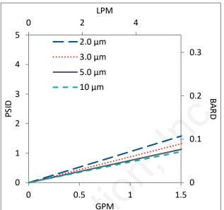
Flow rates for Micro Capsule filters are per filter. The test fluid is water at ambient temperature. Flows are tested using a Micro capsule filter with 1/2" Sanitary inlet and outlet ports. Rates will vary based on end configuration of the Micro capsule.
