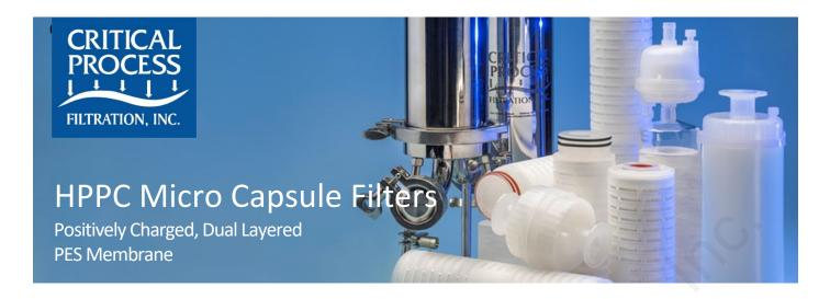
HPPC Micro Capsules are designed for laboratory use with their small filtration area and size. They are made from all the same materials as our larger HPPC filters to ensure consistent results at every scale. These validated, dual-layered PES membrane capsules are well suited for sterilizing products with high particle loads. Final layer pore sizes include 0.03, 0.10, 0.22, 0.45  $\mu$ m.
