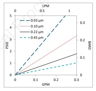
Flow rates for Micro Capsule filters are per filter. The test fluid is water at ambient temperature. Flows are tested using a Micro capsule filter with  $\chi^{\prime\prime}$  Sanitary inlet and outlet ports. Rates will vary based on end configuration of the Micro capsule.
