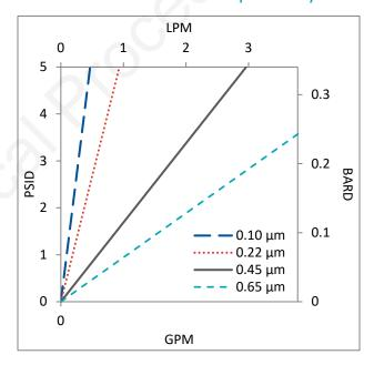
Flow rates for Micro Capsule filters are per filter. The test fluid is water at ambient temperature. Flows are tested using a Micro capsule filter with ½" Sanitary inlet and outlet ports. Rates will vary based on end configuration of the Micro capsule.
