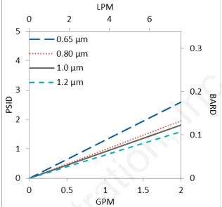
Flow rates for Micro Capsule filters are per filter. The test fluid is water at ambient temperature. Flows are tested using a Micro capsule filter with ½" Sanitary inlet and outlet ports. Rates will vary based on end configuration of the Micro capsule.
